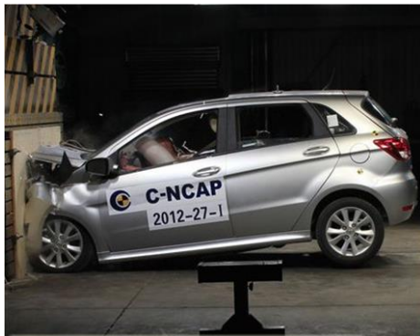
Fig. 4 – Vehicle crash test where engine room is sacrificed (Source:
